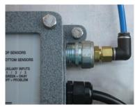
ASA-1 Pressure Switch mounted in ROM Monitor
