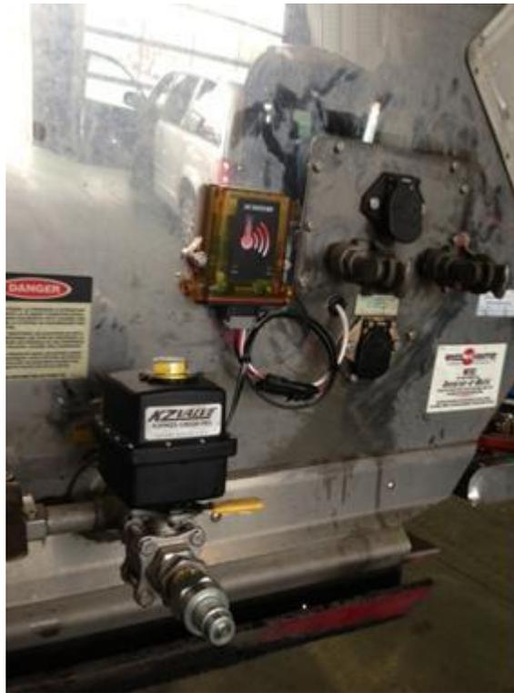
*Figure 18. Mounted Wireless Valve Controller and Ball Valve*
