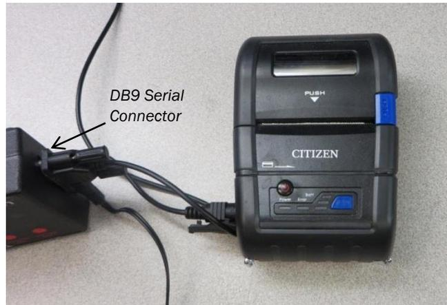
**Figure 4. Printer Connected to In-Cab Display Unit**
