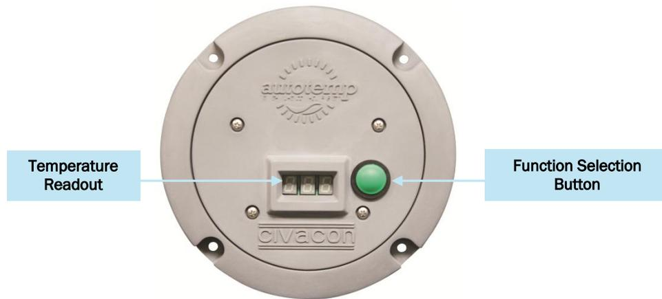
**Figure 8. Temperature Monitoring Unit, Part No. 3602T**
