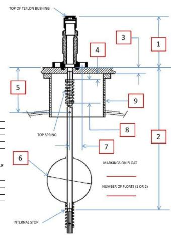
REPLACEMENT GAGE RODS FROM DEVICE DIMENSIONS (USE WHEN ROD IS MISSING)
